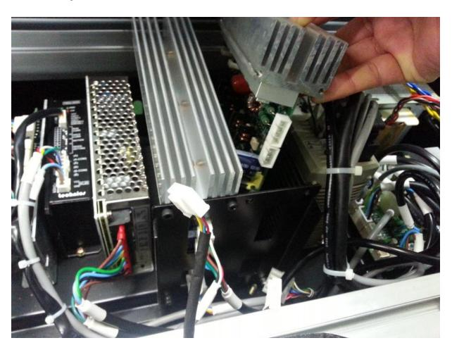
5) Unscrew the Brass Phillip screws to remove the board.
