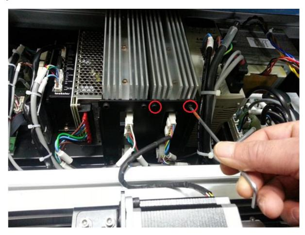
4) Carefully lift the Driver out of the machine.
