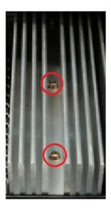
6) Set the new Board and secure to the heat sink with Brass Phillip Screws and carefully reinsert the driver and secure the Allen Screws Re-Connect Cable connections, and place table back in place.
