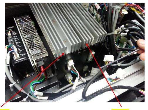
**X-driver** is assembled on left side of heat sinking plate and **Y-driver** is on right Side. Disconnect the connectors to the board you are replacing.
